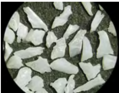
Ceramic grains viewed under a microscope (30X).
