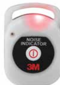
Flashing red at over 85dB(A)
