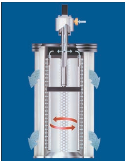
With depth filtration, the harmful substances penetrate the filter medium. A cleaning of the filter is not possible.
