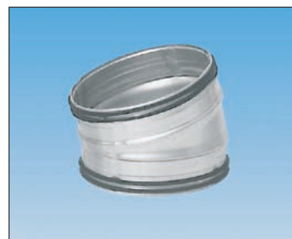
Bends 15° pressed and seam welded. From Ø 250 mm constructed out of segments.
