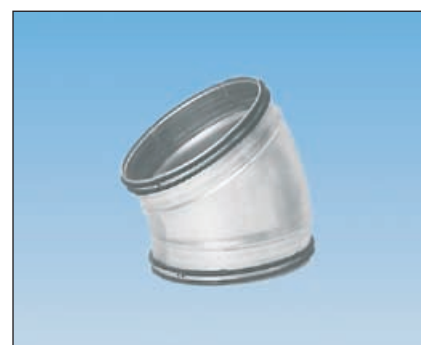
Bends 30° pressed and seam welded. From Ø 250 mm constructed out of segments.
