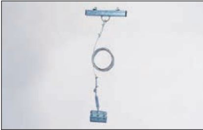
Ceiling fixture with lowering device for C-profile - galvanised, lowering from 1.000 mm to 6.000 mm
