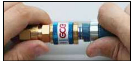
1. Mounting is finished. O-ring is visible.
