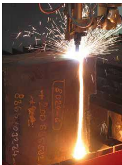
500 mm steel plate cutting
