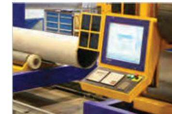
A control unit with touchscreen mounted on the gantry provides all positioning and technology control functions and thus ensures convenient operation of the machine along its whole length.
