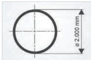
CPCut's cantilever design with open loading area and a powerful chuck enables clamping and processing of pipes and profiles up to Ø 2,000 mm.
