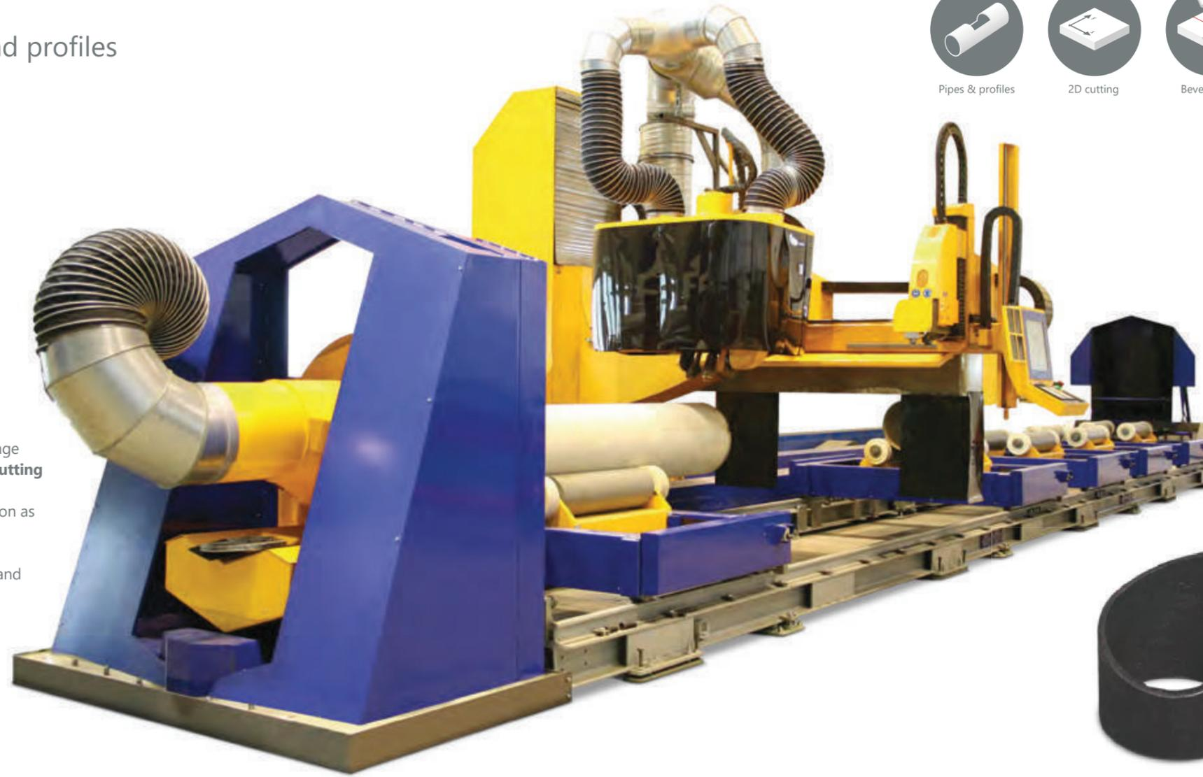
The **CPCut series** offers robust pipe and profile cutting machines designed for processing of a great range of pipe diameters and lengths.
