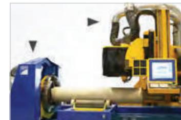
MicroStep's proven suction design for pipe cutting includes direct fume extraction from inside of the pipe through chuck as well as suction from the overhead cover around the cutting head.
