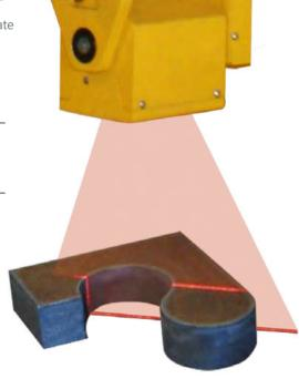
Laser scanner dedicated for scanning of both the contour and position of a straight pre-cut part in ABP feature – additional cutting of bevels for weld edge preparation. ABP technology is available for plasma, laser, oxyfuel and waterjet cutting
