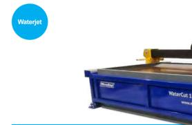
WaterCut is a highly precise and reliable 2D or 3D waterjet cutting machine. Besides a single waterjet tool station, it can be equipped with a multi-tool station with outer span 1200 mm, carrying up to 4 water jets on a single Z axis, or a small drilling unit for piercing of sandwich materials.
