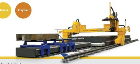
ProfileCut is a machine dedicated for production of steel structures. Besides optional pipe and plate
