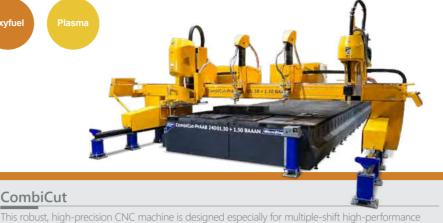
This robust, high-precision CNC machine is designed especially for multiple-shift high-performance plasma and oxyfuel cutting. It allows cutting of steel up to 300 mm thick, bevel cutting with a pair of oxyfuel triple torches or rotators, parallel cutting with up to 8 torches, drilling up to Ø 40 mm, inkjet, micro-percussion or laser marking, as well as pipe and dome processing.
