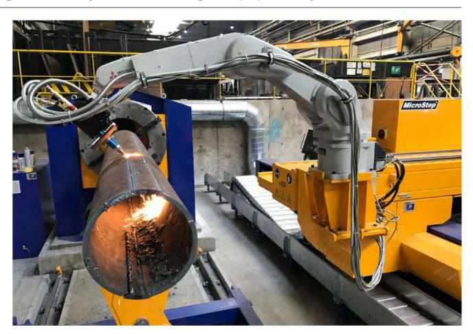
"Furthermore, materials thicker than 25 mm had to be cut with oxyfuel technology which was much slower. MicroStep delivered the complete cutting solution: with a
