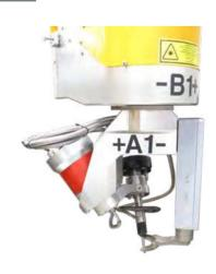
5-axis rotary bevel head for waterjet enables bevel cutting of all types of materials up to 45°. Adaptive taper compensation (ABC) and periodic height sensing (PHS) are included by default.
