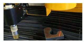
ABP scanner determining the exact position of a part placed on a random spot on the cutting table.
