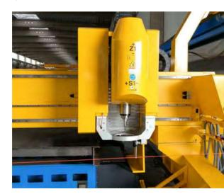
The same gantry can also drill holes with threads, another option to attach formwork elements. "The drilling speed has increased significantly compared to the old system and the fact that we are now able to do the tapping on the same machine is another great advantage," says Winkler.
