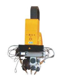
Oxyfuel triple torch with fully automatic gas console enables bevel cutting of V-, X-, Y- and K-cuts with 3 oxy torches within bevel range 20° – 50°. Tilting angle and span of torches can be set manually or automatically.
