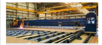
In 2020, the shipyard invested in two panel processing lines which include two 20.5 m wide MicroStep gantries for bevel cutting, primer removal and marking of large-
