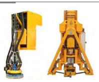
Solutions for removal of thin layer of surface (e.g. primer colour) from plate by shot-blasting or grinding technologies.
