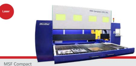
MSF Compact combines precise 2D laser cutting with a compact design. Available in work area sizes of  $1,000 \times 2,000$  mm,  $1,250 \times 2,500$  mm and  $1,500 \times 3,000$  mm, this highly precise machine is particularly attractive thanks to its small footprint. A manually extractable cutting table enables easy and straight-
