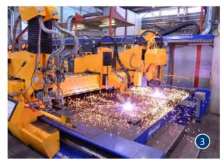
For the company Doppelmayr MicroStep installed a powerful drilling machine of the DRM series 1 and two plasma and oxyfuel cutting machines of the MG series with two gantries 2 + 3 each. The two MG machines are each equipped with a CCD camera 4 for maximum precision when cutting pre-drilled parts.
