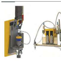
Waterjet tool station for cutting of all types of materials. Multi-tool version can carry up to 4 water jets on a single Z lifter.
