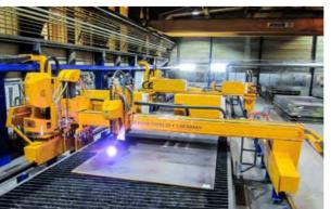
The combined plasma and oxyfuel cutting solution at MAP Prinzing Brennschneidtechnik GmbH enables bevel cutting with plasma, 2D oxyfuel cutting, drilling, tapping and marking on two gantries. At the request of the company, a tool magazine for 16 tools was added.
