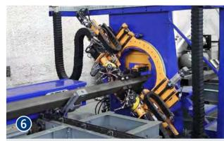
Profile drilling line DS-B allows simultaneous drilling, tapping and marking of rectangular hollow sections up to 12 m long and 300 mm
