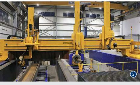
M gantry in EGS equipped with three tool stations. The machine has three work zones: cutting of beams (left) of sheets and domes (front right) and cutting of pipes (rear right)
