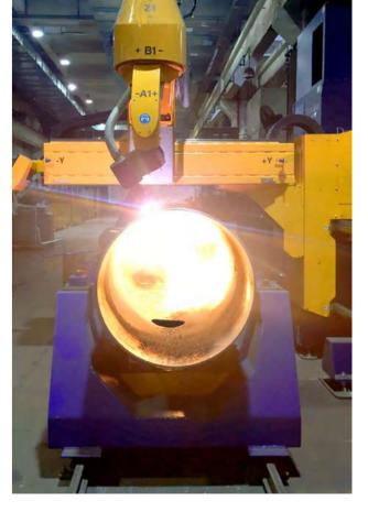
**Top left + right:** Gree's three combined pipe & dome cutting machines from the PipeCut series allow to cut pipes up to Ø 610 mm and a length of 12 m as well as domes up to Ø 1,200 mm. **Bottom left:** Gree Electric Appliances Inc. participated on prestigious projects such as the National Stadium (Soccer City) in South Africa's Johannesburg.
