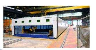
The machine is equipped with a bevel cutting head with 8 kW laser source that allows Chantiers de l'Atlantique to make weld edge and bevel angles up to 45°.
