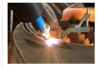
saving of the cutting gas. Higher cutting speeds also mean that there is a smaller heat-effected zone in the material, i.e. better quality of the final part. The necessary additional part handling times with ABP can be offset by having a machine with multiple straight gas torches, and using ABP on multiple parts in one sequence.
