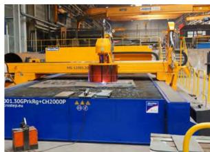
MicroStep delivered the complete cutting solution: with a 12 x 3 m large cutting area for plates up to 150 mm thick and a zone for cutting pipes with a robot situated along the outer side of the machine guides, the machine is capable of processing tubes up to Ø 2000 mm and wall thickness 80 mm.
