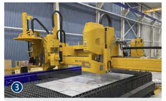
A multi-functional MicroStep machine with drilling up to Ø40 mm (+ tapping and countersinking), inkjet marking and a special plasma bevel head up to 120  $^{\circ}$  tilt angle and endless rotation for plate, pipe
