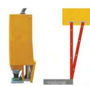
CCD camera can be used for: a) scanning of the shape of template or rest plate for conversion into DXF b) scanning of holes on plate for positioning A laser sensor is used for scanning of plate edges for auto-alignment with the coordinate
