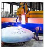
The basic step in production of pressure vessels is precise cutting of dished ends. Automating this process to a high degree while delivering high-precision contours without the need of additional surface finishing provides manufacturers with a clear advantage and saves them a lot of valuable time.
