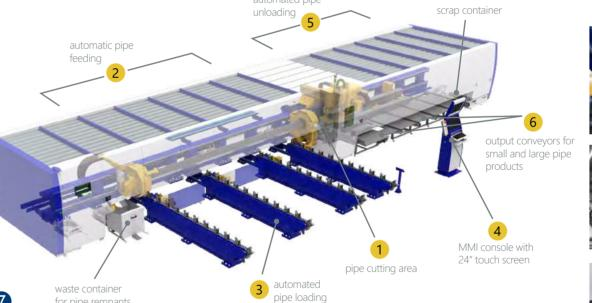
Automated pipe cutting machine MSF Pipe designed for 2D or 3D cutting of round pipes up to 6 m length and diameter Ø 200 mm as well as for tubes of rectangular and other cross-sections. The machine features a laser scanner that is used to determine the real shap of pipes to be cut to ensure accurate cutting results.
