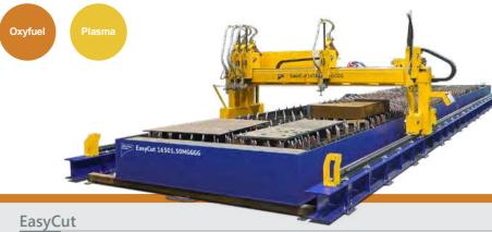
The EasyCut series stands for modern oxyfuel cutting at the highest level. It is the ideal system for precise and cost-effective oxyfuel cuts up to 300 mm and impresses with its robust, simple and mainte-
