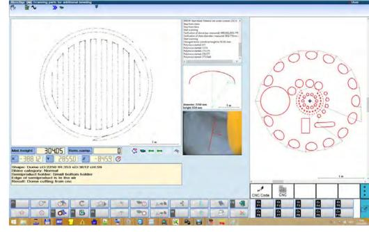
Thanks to the mScan technology, the 3D scan of a dome enables to determine production-related deviations from the ideal contour that then could be compensated for accordingly during cutting.
