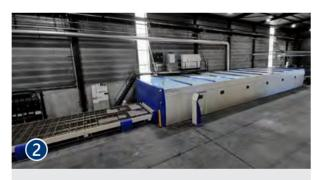
Large-scale fiber laser bevel machine MSF Pro with work area 16
