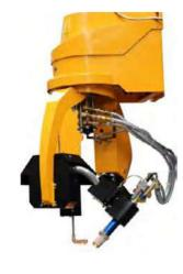
5-axis rotary bevel head with endless rotation enables oxyfuel bevel cutting of plates, pipes and profiles up to 60°. The innovative ITH torch holder includes sensors for torch displacement detection, IHS and auto-calibration.
