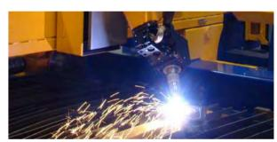
With beveling technology from MicroStep, V-, Y-, and (under certain conditions) also X- and K-cuts can be added to already pre-cut parts.
