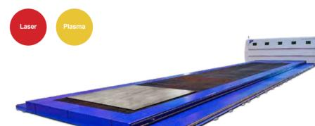
MSF Pro is a powerful fiber laser cutting machine designed for the production of highly accurate parts at high cutting speeds, with surprisingly low maintenance and operational costs. The machine is equipped with an automatic shuttle table up to the size of 15,000 x 3,000 mm. The optional equipment includes pipe and profile cutting, and drilling, tapping and countersinking.
