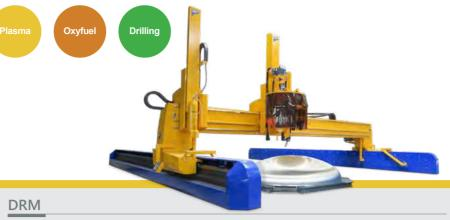
DRM is a heavy-duty CNC cutting machine designed for a wide range of dome, plate and pipe cutting applications. Its robust gantry allows a vibration-free operation of heavy equipment such as automatic oxyfuel triple torches or a 120° rotator with Z-axis stroke 1,500 mm for cutting of dished ends. DRM can be delivered also as a high-performance drilling machine with special drilling table.
