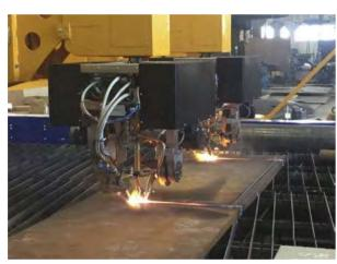
Oxyfuel triple torches make K-cuts in one go but lack the ability to cut really thick
