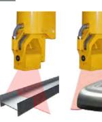
Laser scanner with a rotation and tilting ability allows to create detailed surface representations of scanned objects - e.g. profiles and domes. In combination with mScan technology it allows to adjust cutting plans according to true shape of 3D
