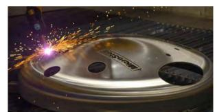
machine gives them the ability to cut 7.5 x 4 m plates along with domes of up to Ø 3,000 mm in two separate work zones.
