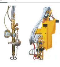
Oxyfuel tool station with manual tilting possibility up to ±45°. Fully automatic gas console with preset parameters ensures stable quality of cuts and best efficiency. Multi-tool version enables stripe cutting with stripe width  $\geq$  70 mm.
