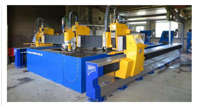
proved to be no longer adequate because operation and loading took too much time and limited the production. And so, Striegel considered several offers for new equipment and eventually decided to invest into a combined CNC waterjet-plasma cutting machine from MicroStep. "I made that decision because I had good experience with MicroStep."
