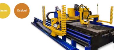
DRM Max machine has a dedicated drilling/milling area with an independent sub-gantry and two powerful retainers that make milling up to a length 750 mm along the X axis possible. The robust design enables drilling up to Ø 70 mm and a variety of milling jobs such as large hole milling, face milling, pocket & slot milling, chamfer milling, thread milling or counter boring.
