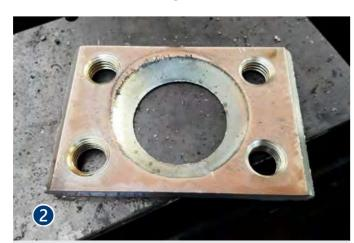
Hardox part drilled, tapped and bevel cut with plasma on a MicroStep DRM
