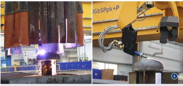
f a smaller dome with plasma (left) and oxyfuel (right). The machine can cut domes up to a diameter of Ø 2,000 mm and a heigh
