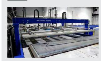
the middle pallet with MSLoad system, with a stockpile of unloaded orders in the front.
