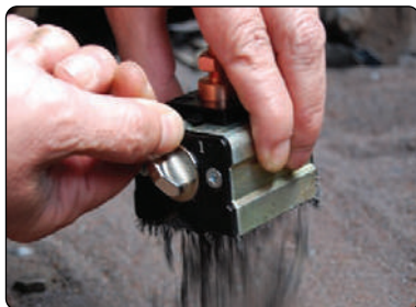
Turn OFF the PowerBase™ Grounding Magnet and metal chips fall away.
