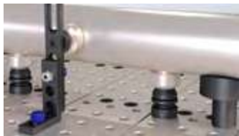
Vertical application using Locating Post + V-Block Spacer
